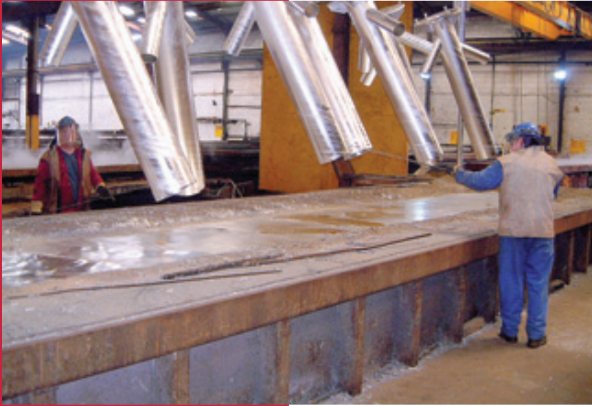
Hot dip galvanising tank in action
